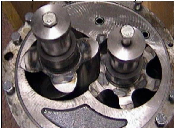
Insufficient cooling led to thermal expansion of the rotors, which came in contact with the housing.
