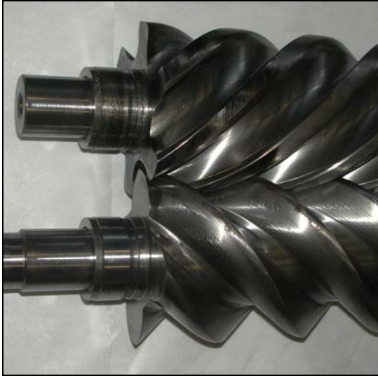
Visible traces of dirt on the rotors and inner bearing ring.
